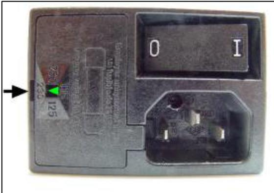
Insert a screw driver (3 mm) into the groove and press in the direction of the rear panel. The insert then comes off its mounting and can be pulled out easily.
